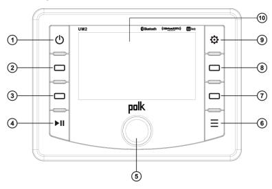
Press the **Mode** button (6) to enter mode selection display. Press the **SiriusXM** soft button (8) to change to SiriusXM mode.
